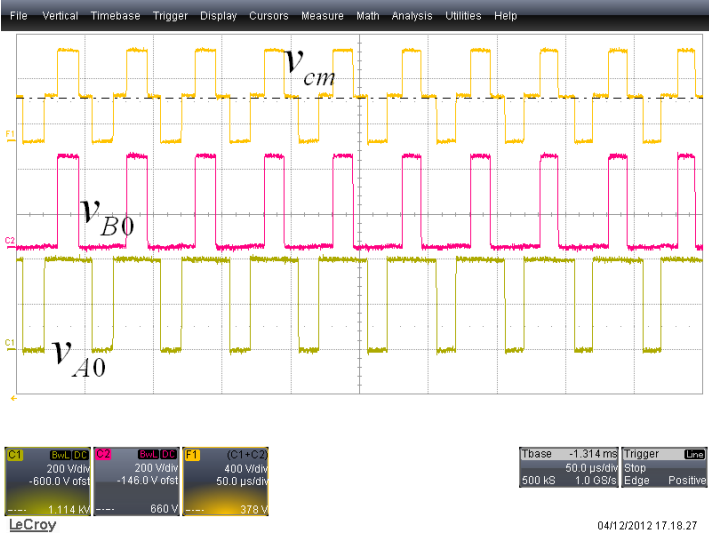
Figure 4.41: Common mode voltage at the output of the converter in case of unipolar PWM.
