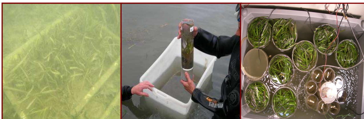
Figure 5.2. From left to right: acclimatization on the river bottom, microcosms collection, incubation system in laboratory.
