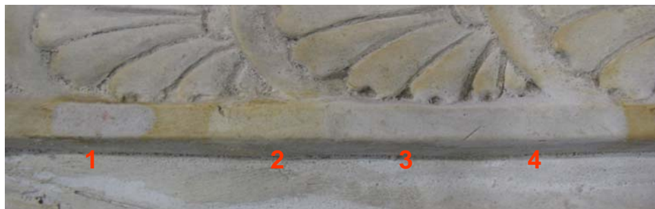
Fig. 14 cleaning testing performed with cotton-swab (1), and Agar gel for 5 min (2), 20 min (3) and 30 min (4)
