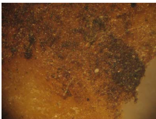
Fig. 45 Stereomicroscopical image (70x) of the surface CVE1 sample from Il Velo . The surface seems very heterogeneous.
