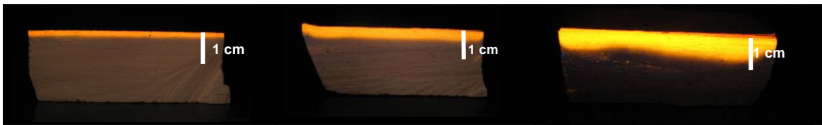
Fig. 24 cross-sections of plaster treated with agar 3% for 3 min, 20 min, until dry out of the gel (from the left to right) under Uv light. Water was tinted with rhodamin
