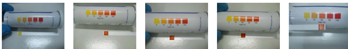
Fig. 25 calcium test of gel (from left to right) before treatment and after 3 min, 20 min, until dry out and application of cotton swab
