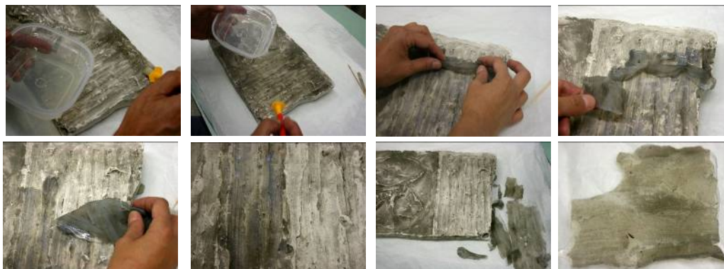
Fig. 9 Mode of preparation, application and removal of Agarose-based gels onto plaster surface.
