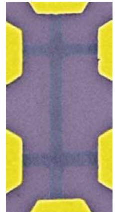
Figure 16. SEM micrograph of a graphene (dark violet) device for Hall measurements.
