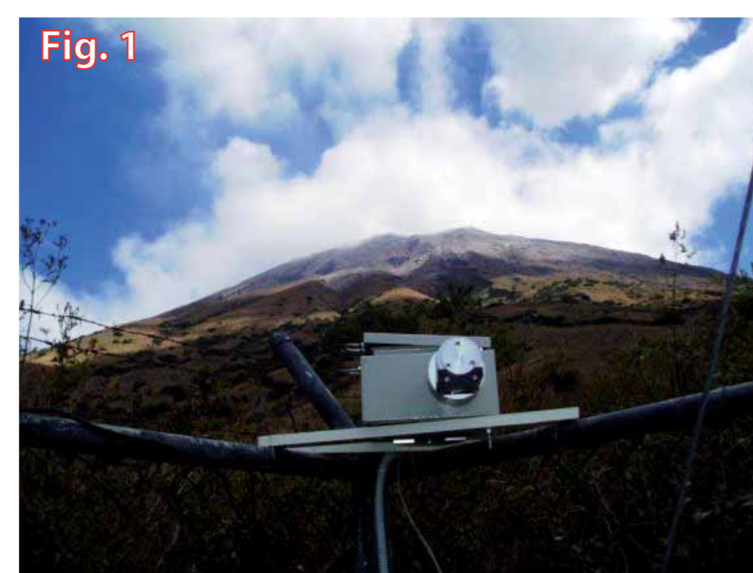
Fig. 1 A view of Chaparrastique Volcano behind the scanner spectrometer FLAME (Flux Automatic MEasurements) installed at Lacayo site.
