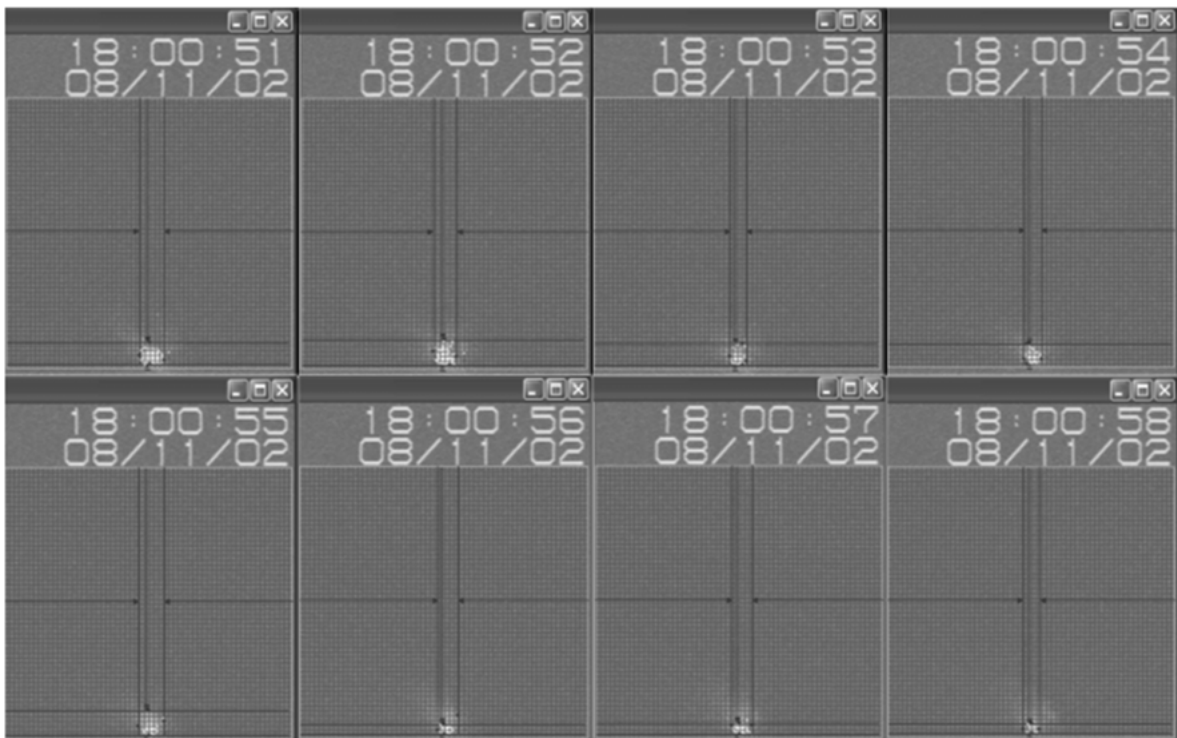
Figure 4. A frame sequence processed by the analysis tool. As can be observed in Figure 2, the analyzed event has been classified as an explosion with an aspect ratio of 1.07.
