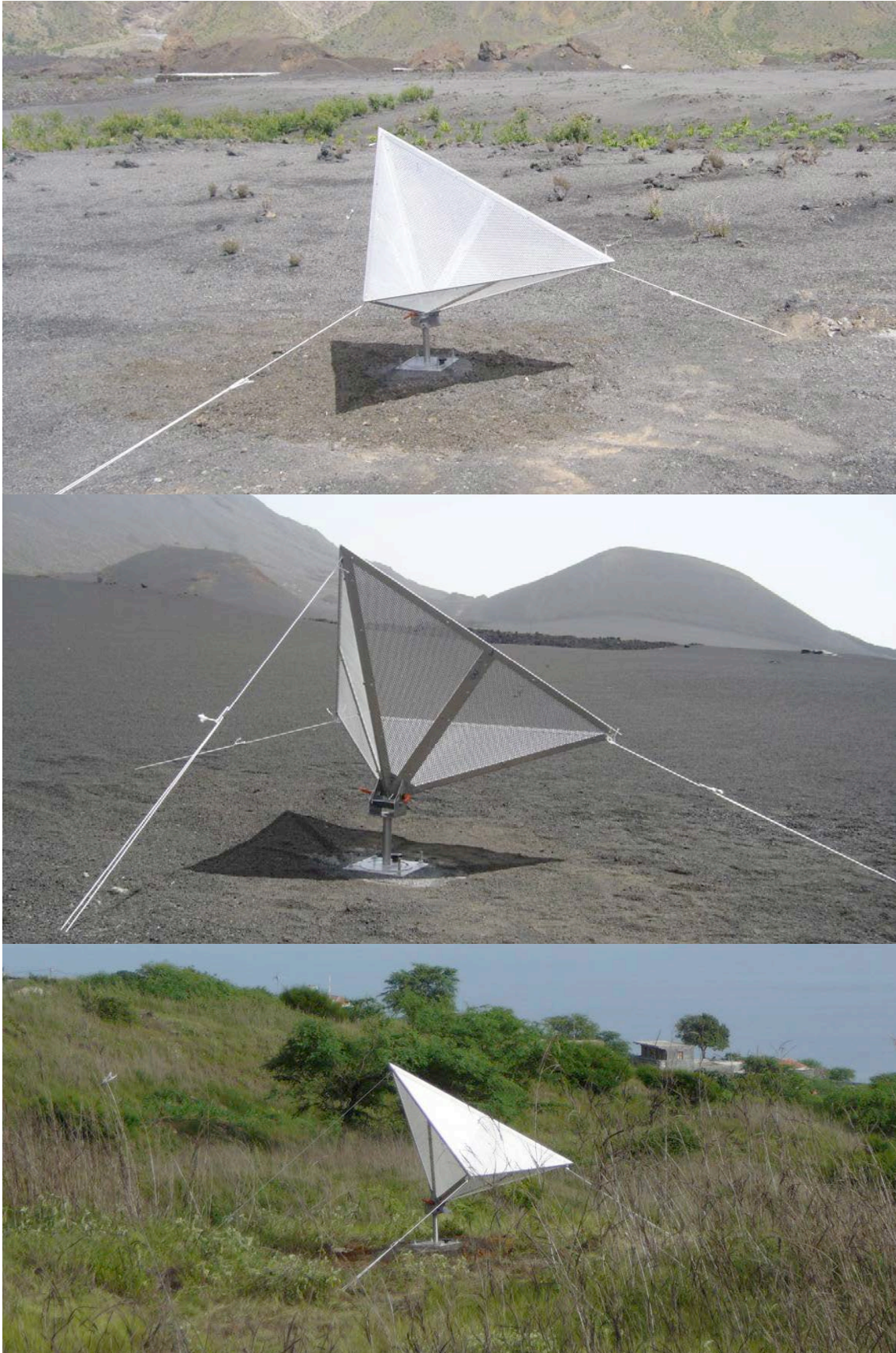
Figure 6. The three CRs successfully installed. Upper, middle and bottom images refer to the two CRs close to Chã das Caldeiras and the one close to Fonte Aleixo, respectively.
