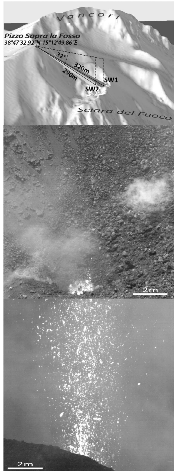
Figure 1. (top) Southward view of the field setup for the high-speed filming experiments at Stromboli volcano. The camera, located at Pizzo Sopra la Fossa and tilted downward by 32^\circ , looks at the 320- and 290-m away SW1 and SW2 vents. Representative still-frames of (middle) a meter-sized bubble bursting at the surface of SW1 vent and (bottom) a well-collimated ejection jet at the beginning of an explosion at SW2 vent. Incandescent pyroclasts are in white, clearly distinguishable from darker (colder) surroundings.
