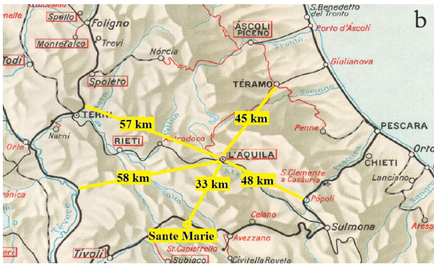
Figure 3. (a) Railway map of Central Italy. The DC electrified railway line that mainly interferes with L'Aquila Geomagnetic Observatory is Roma-Sulmona-Pescara in light blue colour; at the contrary the Terni-L'Aquila-Sulmona line, in green, it does not disturb the magnetometers because is not electrified (diesel power). (b). Minimum distances of L'Aquila Geomagnetic Observatory from the nearest DC electrified railways (Sante Marie station is the nearest one at 33 km). The railway line that contributes most to the noise at L'Aquila observatory is that from Sante Marie to Popoli, in particular from Avezzano to Pescara in the flat Fucino (Marsica site) due to the high electrical conductivity of lacustrine sediments and clay deposits in the subsoil; in fact the wide basin of Fucino until 1875 was a lake, the third largest of Italy. (c). Geological map of Abruzzo [Vezzani and Ghisetti 1996]: the position of L'Aquila observatory is indicated in the upper left by the red point. In the bottom center the position of Fucino is represented by light blue color and with similar color the Peligna Valley in the lower right.
