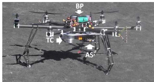
Figure 1. Hexacopter UAV system: the locations of battery pack (BP), thermal camera (TC) and acquisition system (AS) are shown.
