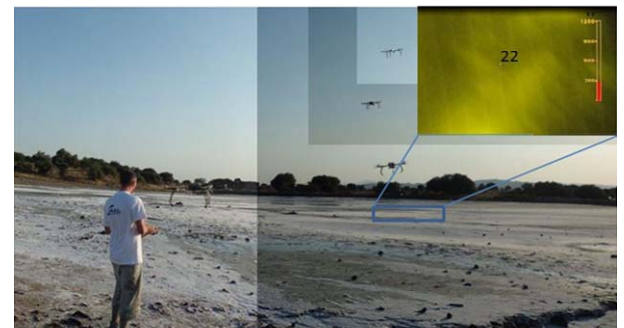
Figure 6. The frame composite visible image shows the reconstructed pattern of the second hexacopter flight. Inset shows the frame from the drone-borne thermal camera taken on the same site as field temperature measurements and the temperature measured in the centre of the image.
