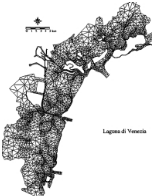
Fig. 2 - Finite element grid of the Venice lagoon.
