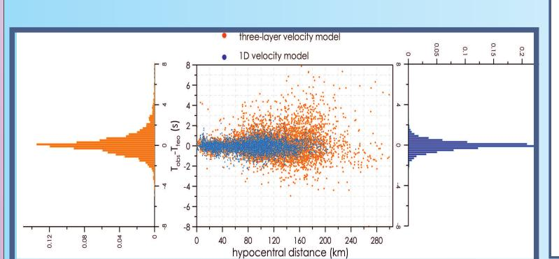
Figure 8. Plot of residuals between observed and theoretical travel times, and their histograms. Orange points refer to the three-layer velocity model; blue points refer to the minimum 1D velocity
