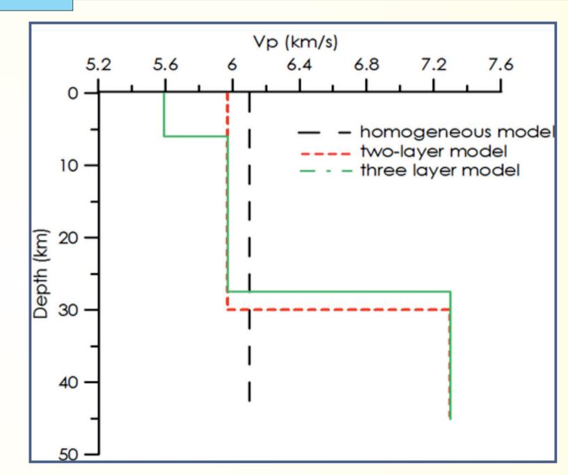
Figure 6. The layered Vp velocity models obtained with the grid-search method.
