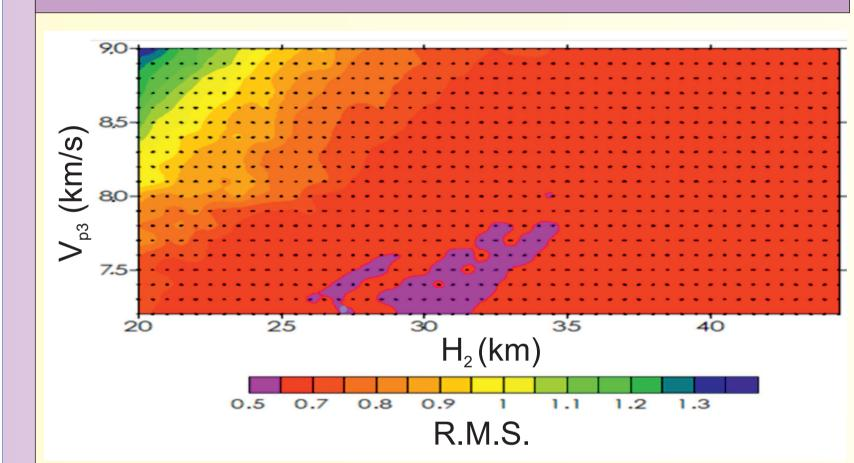
**Figure 5.** RMS plot in five-dimensional  $(V_{p1}, V_{p2}, V_{p3}, H_1, H_2)$  parameter space:in particular, V<sub>13</sub> vs H<sub>2</sub> is shown. Each point corresponds to an autput of HYPO71, related to the initial parameters: a fixed Vp/Vs ratio to 1.8, a tryal depth ranging from 20 km to 45 km and a tryal Vp ranging from 7 km/s to 9 km/s.
