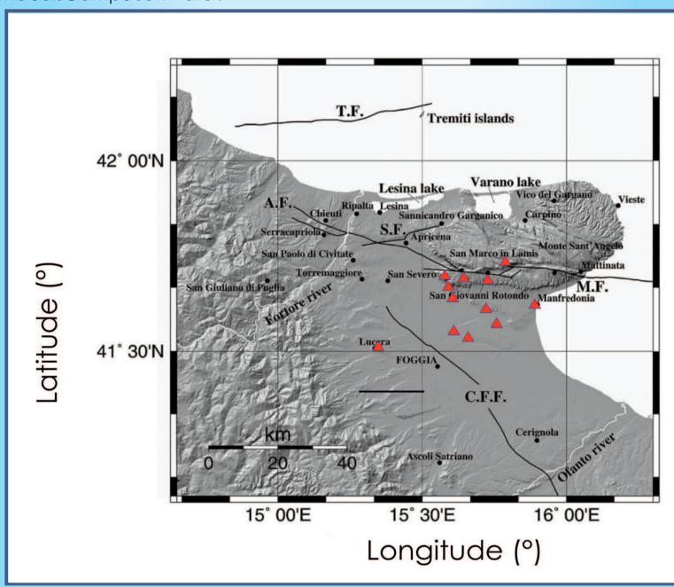
Figure 2. Location of the seismic stations of the Otrions seismic network. A.F: Apricena fault; M.F: Mattinata fault; T.F:Tremiti fault; C.F.F: Cerignola-Foggia fault; S.F: Sannicandro Garganico-Apricena fault (redrawn from Del Gaudio et al., 2007).
