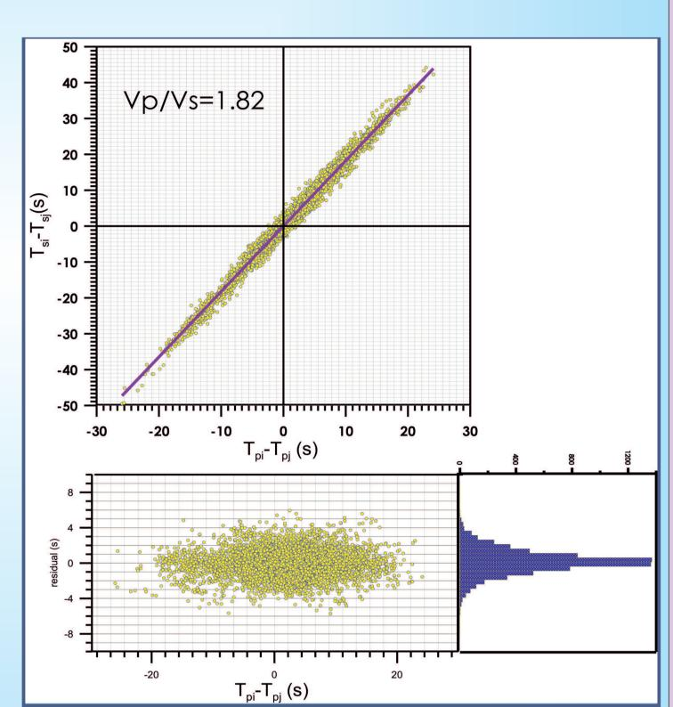
Figure 4. Modified Wadati diagram(Chatelain, 1978) (on the top) and residuals on S wave travel times (on the bottom).
