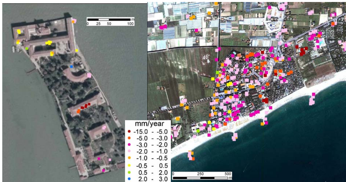
Fig. 4. Displacement rates from IPTA at the San Servolo island (left) and along the Cavallino littoral (right) averaged over the 2003-2007 period. Negative values mean subsidence
