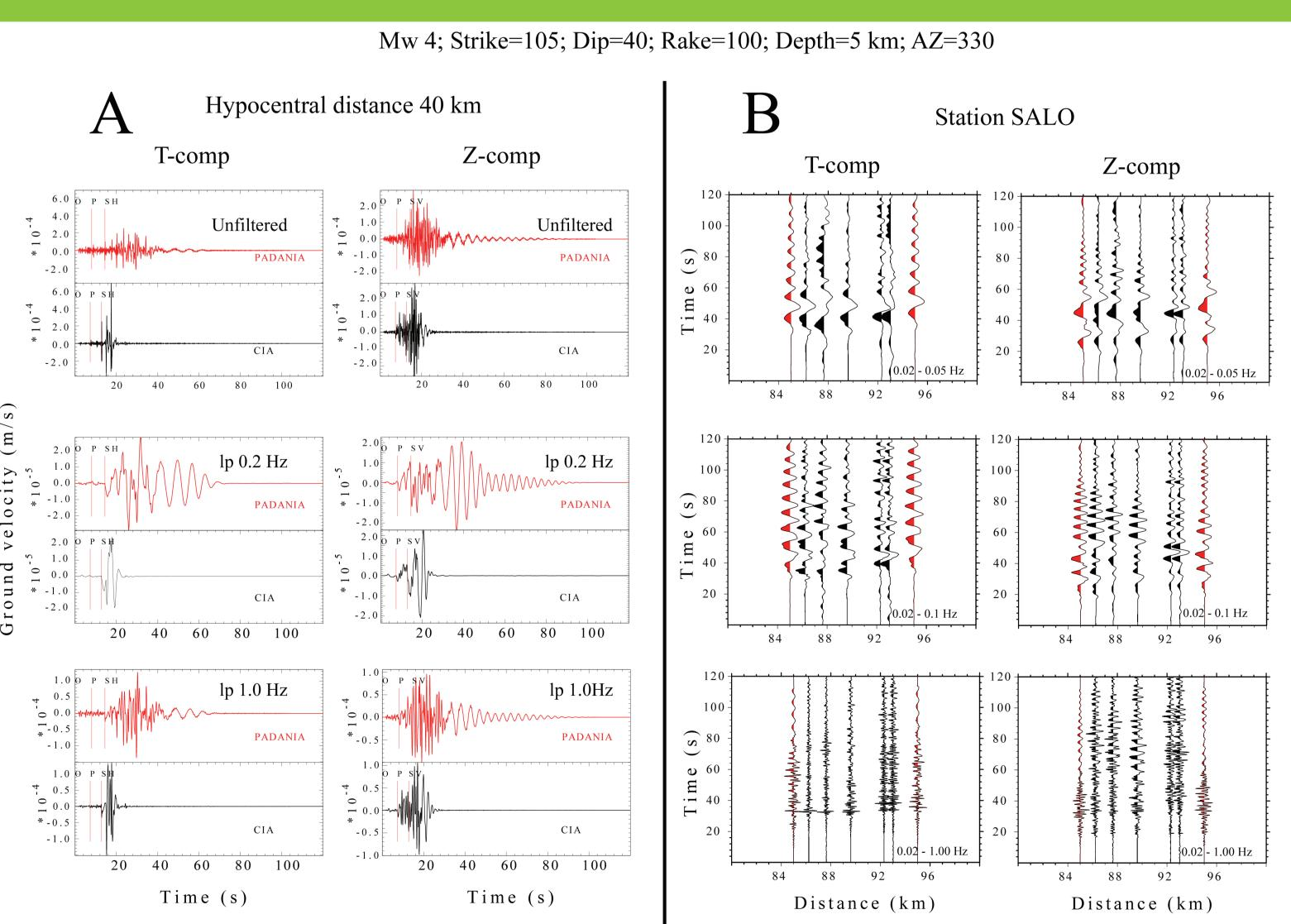
(a) Synthetic seismograms (left: transverse components; right: vertical components) calculated at 40 km distance and at an azimuth of 300° over the PADANIA and CIA crustal models (red and black, respectively), for an earthquake of Mw 4, strike =  $105^{\circ}$ ; dip =  $40^{\circ}$ ; rake = 100°. From top to bottom: i) unfiltered; ii) bandpass filtered between 0.02 and 0.2 💩 Hz; iii) bandpass filtered between 0.02 and 1.0 Hz.
