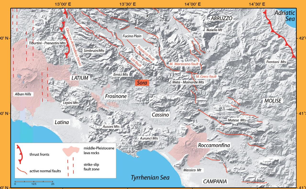
Figure 1. Map of the SLAM study area with the main tectonic-structural elements
