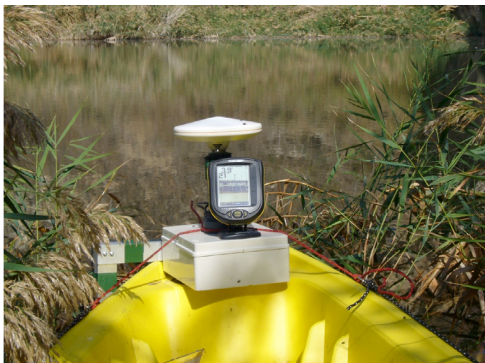
Figure 3. Particular of the bow of the kayak used for the surveys with GPS antenna and echosounder; the sonic transducer is mounted at the submerged end of the metal bracket on the left of the instrument.
