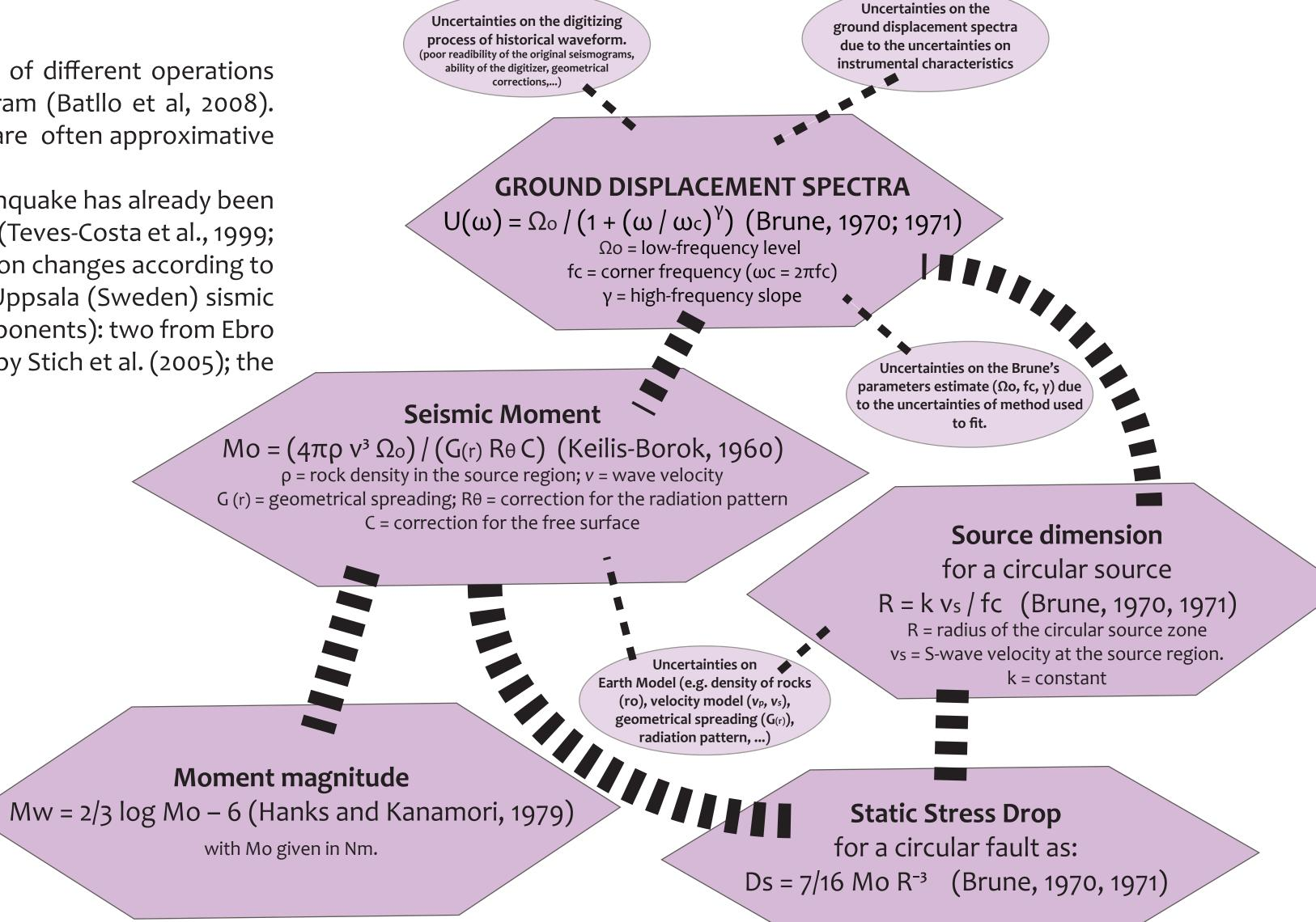
Sismic parameters (exagonal boxes) estimated using our approach and uncertainties sources (ellipsoidal boxes) that influence the different steps of computation. The formulas inside the boxes are those used for computations. The increase of the thickness of the dashed lines has the purpose of graphically display the variability of the uncertainties associated with each step of the process and that are propagated in the final results of the analysis.
