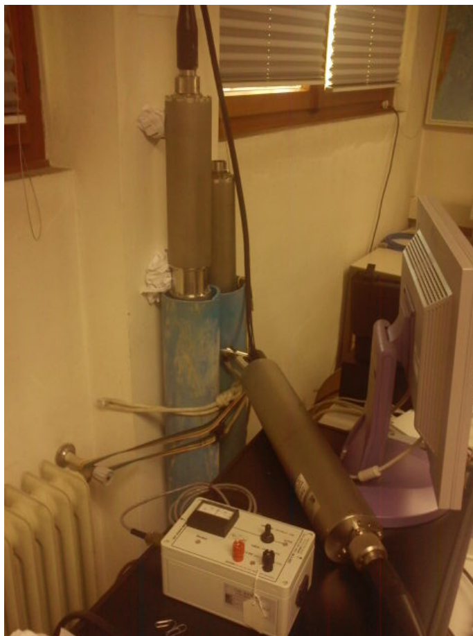
Figure 2 – Guralp CMG-3T/5T borehole sensor with DM24 digitizer and control box
