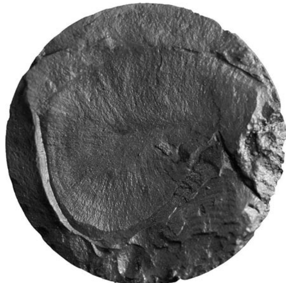
Fig. 5 – Photograph of subhorizontal fracture at 964.03 mbsf in the AND-2A core with hackle plume demonstrating induced, tensile fracture origin. Core is 6.1 cm in diameter.
