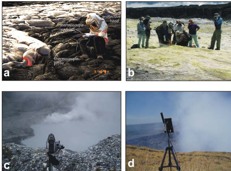
9 10 Fig. 1. Different modes for temperature and volcanic gas sampling. Conventional in situ 11 measurements of (a) the temperature of Hawaiian pāhoehoe lava flow fields (photo by P. 12 Mougini-Mark, volcano.oregonstate.edu), and (b) volcanic gas from the summit fumarole 13 field of Kīlauea volcano in 2005. In (c) and (d) ground-based thermal imagery of the Laguna 14 Caliente crater lake (Poás volcano, Costa Rica; 2009) and UV-DOAS measurements of the 15 Santiago crater (Masaya volcano, Nicaragua; 2009) volcanic plume, respectively.
