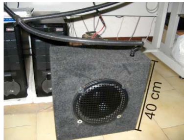
Figure 3. Picture of the subwoofer used for the tests. Note the plastic hose connected with the enclosure.
