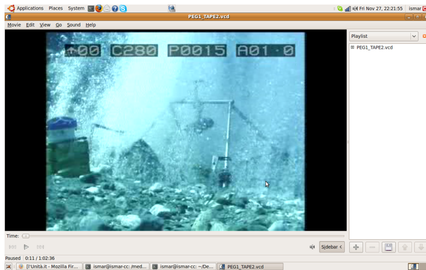
Figure 4: September 2003 flux-measurement experiment: the ADCP and rotor current meter (within gas, on the frame) are visible.
