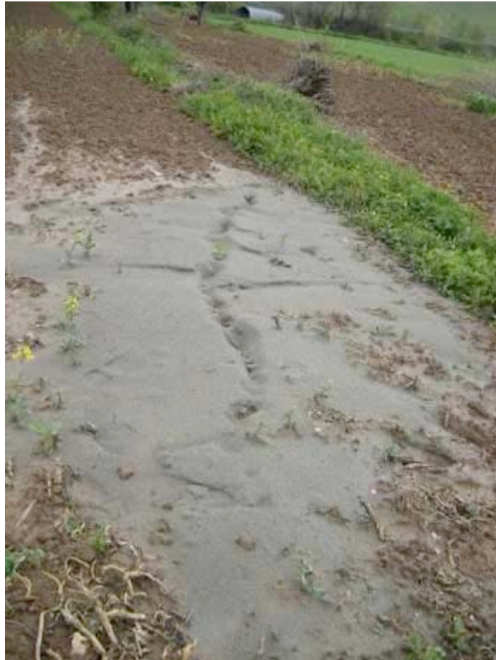
Figure 6. Sand boils observed at Vittorito, produced by the L'Aquila earthquake of 6.04.2009 [ http://www.rete5.tv/images/stories/Ambiente/vulcanetti.jpg ].
