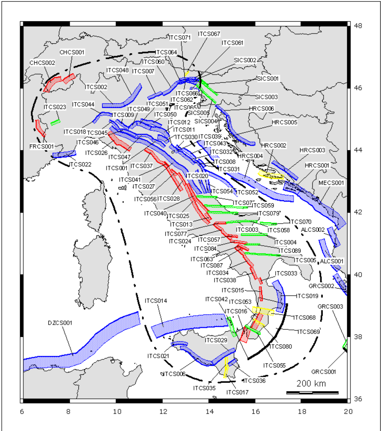
Figure 11. Map of the CSS from the DISS version 3.1.0 database (DISS Working Group, 2009), classified according to faulting mechanism. Red, normal (NN); blue, reverse (RR); green, right-lateral (RL) strike slip; yellow, left-lateral (LL) strike slip; black, subduction. Bold line, top edge of fault; patterned, vertical projection of fault to the ground surface; dashed line, the study area
