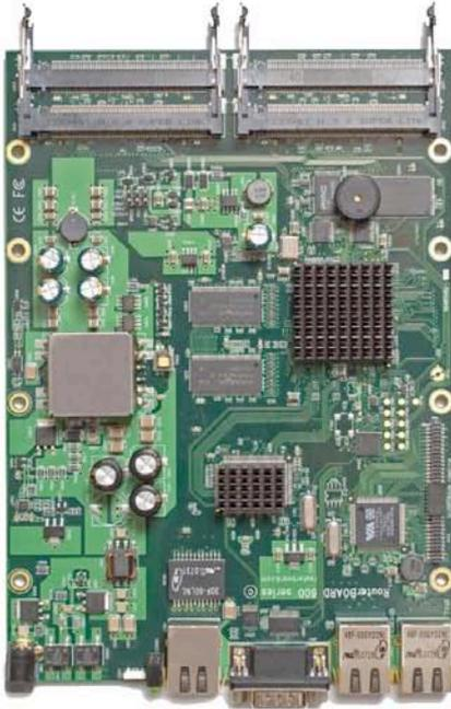
The high performance wireless platform. It has four miniPCI slots and three gigabit ethernet ports and it is the fastest wireless board that MikroTik has ever made.
