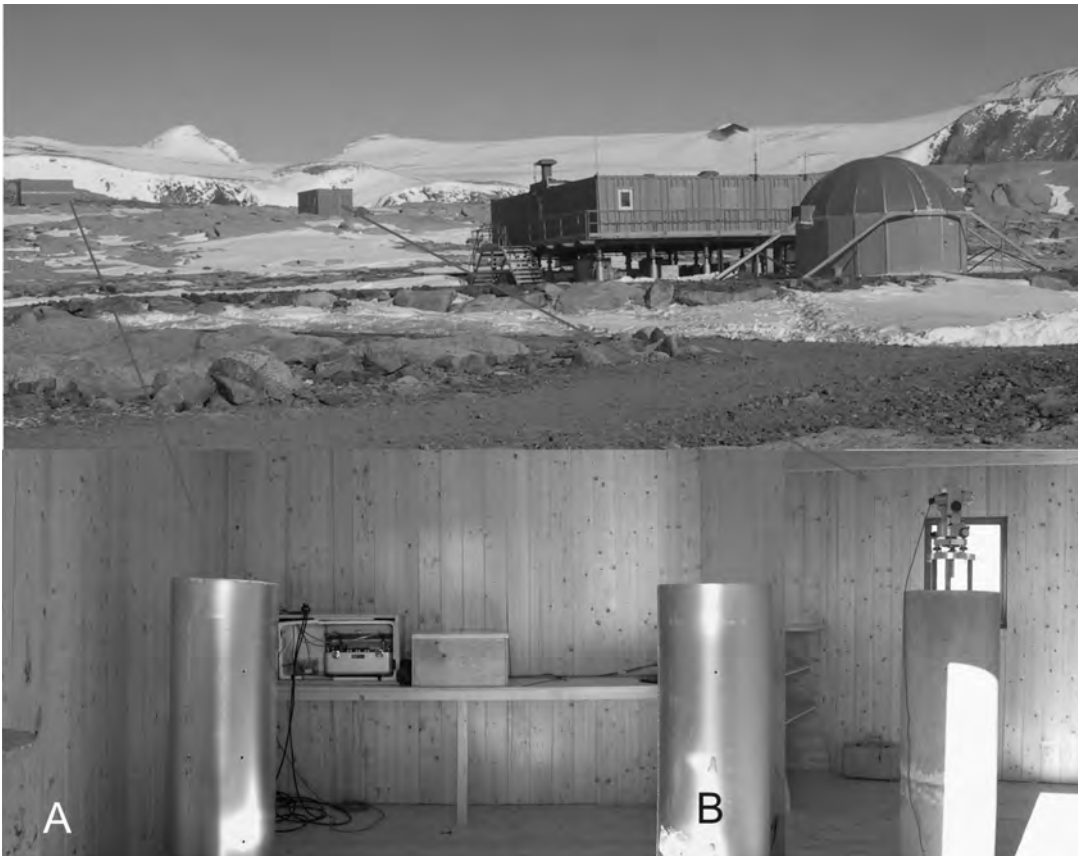
Fig. 1a,b. Geomagnetic observatory at Mario Zucchelli Station: a) variometer shelter; b) absolute measurement shelter.
