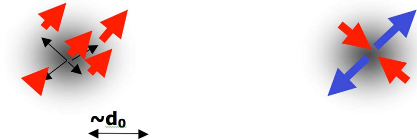
Figure A3: Example of strain rate calculation. On the left figure five sites are present: one is at the centre of a circle of radius equal to the typical correlation length of the ensemble of velocities, and four additional velocities are uniformly distributed about that point within the circle. On the right we have the corresponding strain rate eigenvectors. The structure of the velocity distribution is such that one expects an extension in the NE – SW direction. This deformation regime is then a mean property of the entire circular area.
