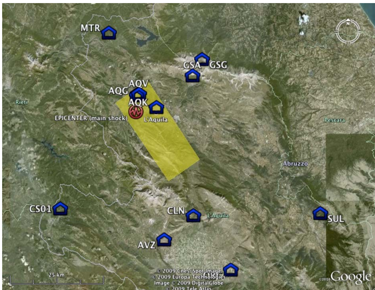
Figure 12 - Locations of accelerometric stations in Abruzzo region that recorded the 6 April 2009 main shock and of a preliminary fault plane surface, shown in yellow.
