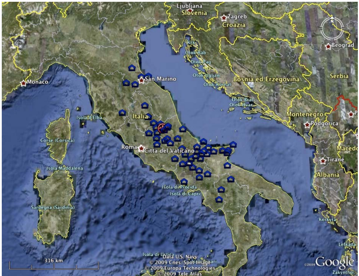
Figure 15 - Locations of instruments that recorded 6 April 2009 mainshock.
