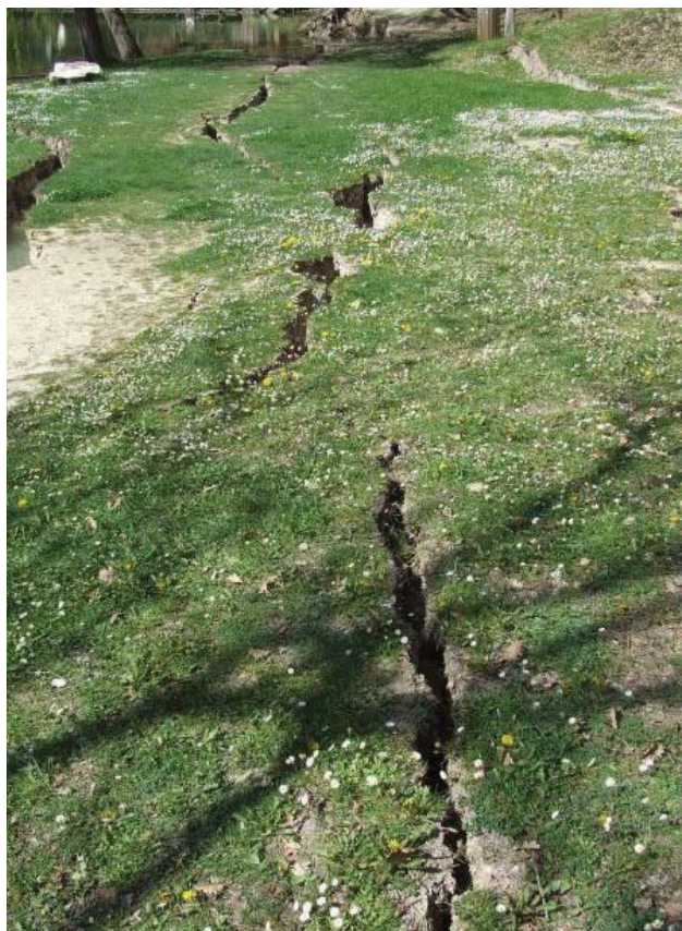
Figure 56 e 57 Fratture beanti sul bordo settentrionale del lago Sinizzo, WPT MT5 42.2913/13.5760. Figures 56 and 57 Open failures on the northern bank of the Sinizzo lake, WPT MT5 42.2913/13.5760
