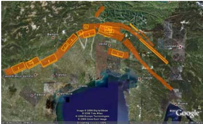
Fig. 2 – Overview of the seismogenic sources of northeastern Italy and western Slovenia included in DISS 3.0.4. The Individual Seismogenic Sources are represented with yellow rectangles, Composite Seismogenic Sources with red ribbons.
