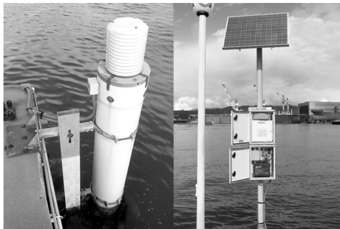
Figure 4. Instrumentation of RMN La Spezia station: ultrasound hydrometer and tide gauge (on the left), and acquisition station containing the barometer (on the right).
