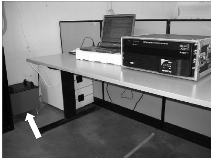
Figure 10. The Newtonian acquisition station. The arrow indicates the gravity sensor.
