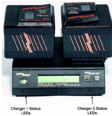
Figure 5. a) Battery charge unit and b) led description.
