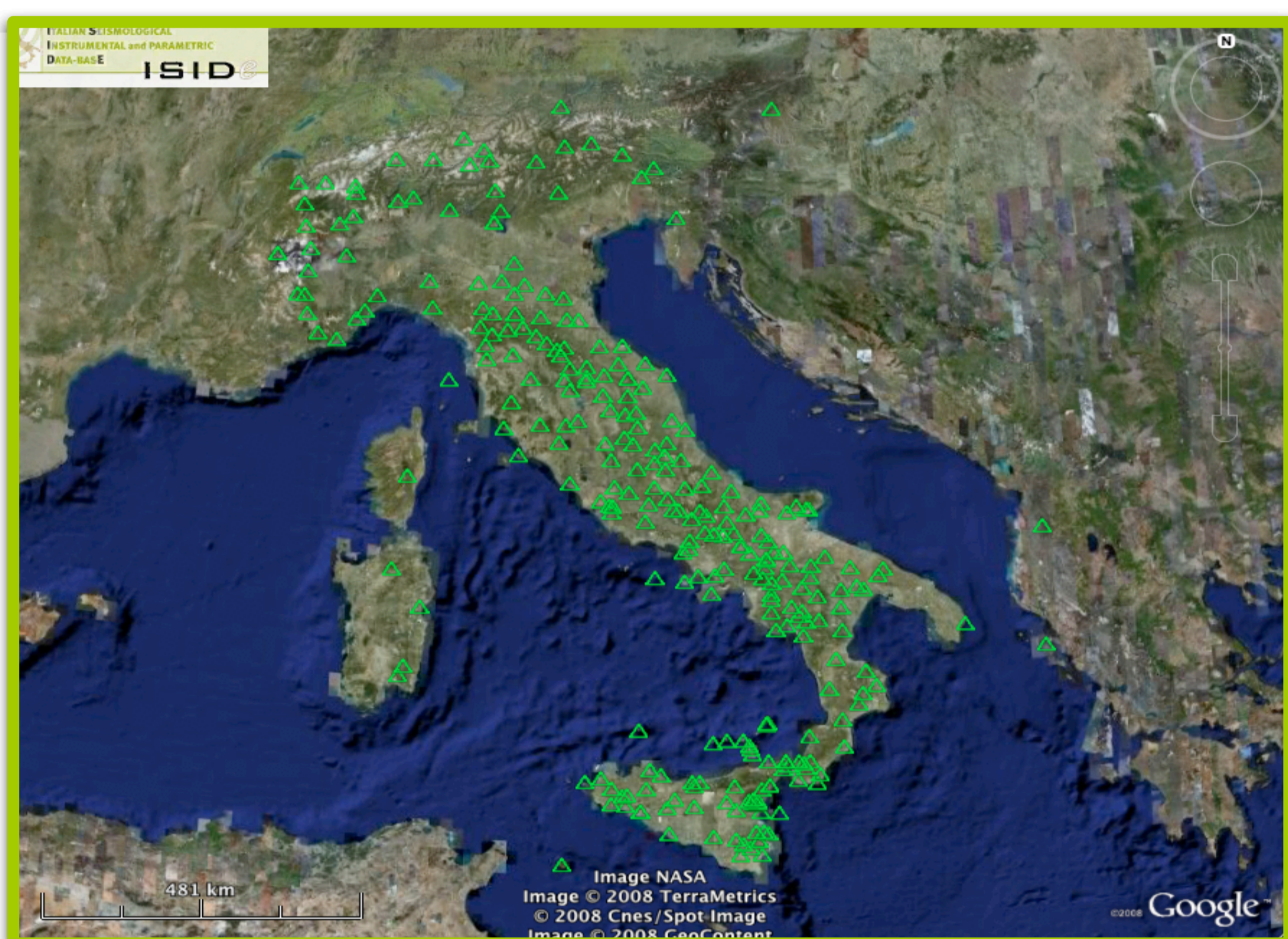
Figure 2 | Stations joining the Italian Seismic Network monitoring system. The National Earthquake Center of INGV collects in Rome seismograms in real time from about 250 velocimeters (640 channels).
