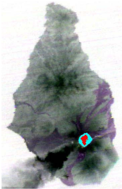
Figure 7. Soufrière Hills (Montserrat) - High spatial resolution surface thermal anomalies product obtained by processing TERRA-ASTER data (2006-02-19). Red points identify high temperature anomalies, blue points identify low temperature anomalies (Lava dome).
