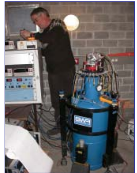
Figure 3: The last Compact Tidal SGs, manufactured by GWR Instruments (San Diego) during its set-up by the manufacturer (R. Warburton) in Walferdange (Luxembourg). The sensor uses a Nb superconducting test mass which is levitated in a magnetic field created by superconducting coils. The extremely low noise and low drift are primarily due to the operation of the components at liquid He temperatures regulated to a few micro-Kelvin inside a vacuum can. A special refrigeration unit allows the instrument to be run indefinitely with only one filling of liquid He.
