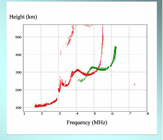
The existence of earth magnetic field makes a second path possible being it the extraordinary trace.
