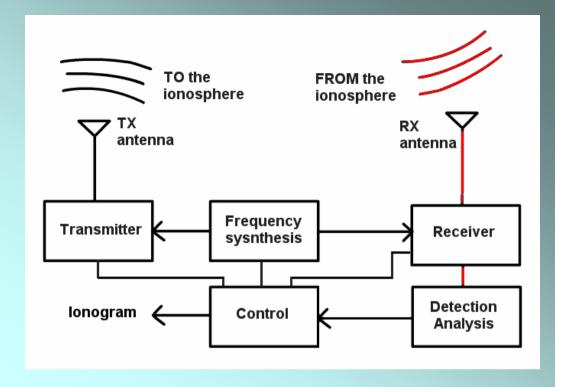
**Control system**: enables the TX to emit energy and, after that, enables to receiver starting the so called "listening time".
