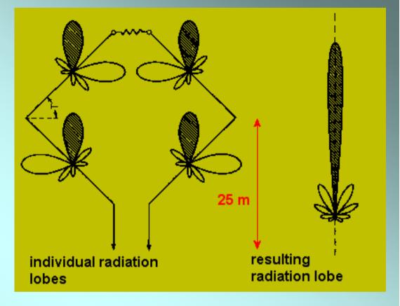
Each side of the antenna is a resonating element; the resistive load at the top is added to widen the band.
