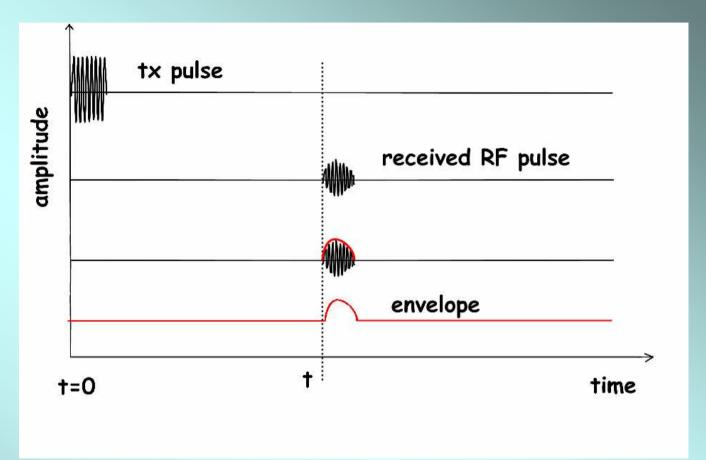
The early model of radars were based on the envelope technique.
