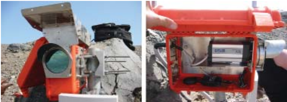
Fig. 5. Polycarbonate box containing the A 40 M FLIR thermal camera.
