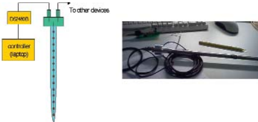
Fig. 1. Left: extremely simple electrical wiring: just paralleled devices. Bottom: a look of the prototype head.
