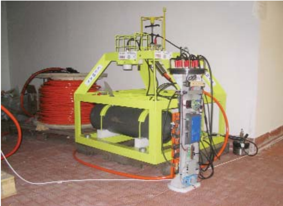
Fig. 2. The fully equipped CUMAS set-up in the laboratory during tests; the acquisition system was kept out of its frame temporarily to check on its operation.
