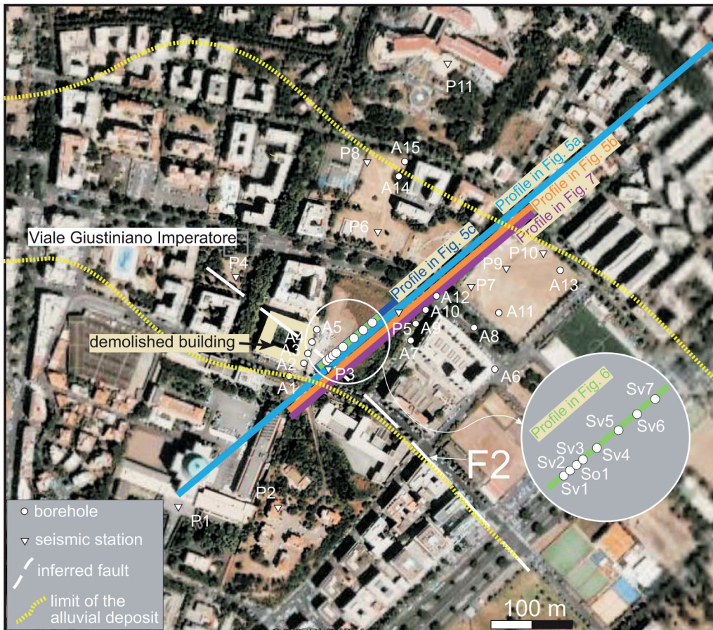
Fig. 3. Location of the geoelectric profile (blue line) and of the boreholes campaign performed in this study (Sv1-Sv7, So1, see the enlargement in the circle). The setting of the INGV seismic stations (P1-P11) at the Grottaperfetta valley and the location of boreholes whose logs were acquired from different sources (A1-A15) are also shown.
