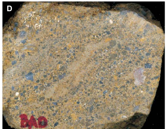
D Handspecimen of a lapilli tuff from Badacsony that is unsorted, matrix-rich and having volcanic glass shards with different shape and vesicularity. The matrix is rich in quartzofeldspathic-origin minerals and rock fragments. The short side of the photo is about 10 cm
