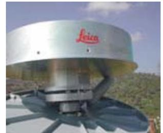
**Figura 7** Antenna Choke-Ring AT504
