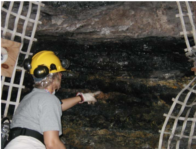
Figure 5 Sulcis coal stratification (Produttivo Formation): alternation of coal strata and carbonaceous-clays, above the “Miliolitico Limestone Formation”, under the coal strata, seat of the SUL 4 groundwater sample.
