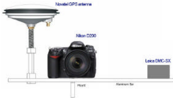
Figure 5: Physical arrangement of Backpack components.
