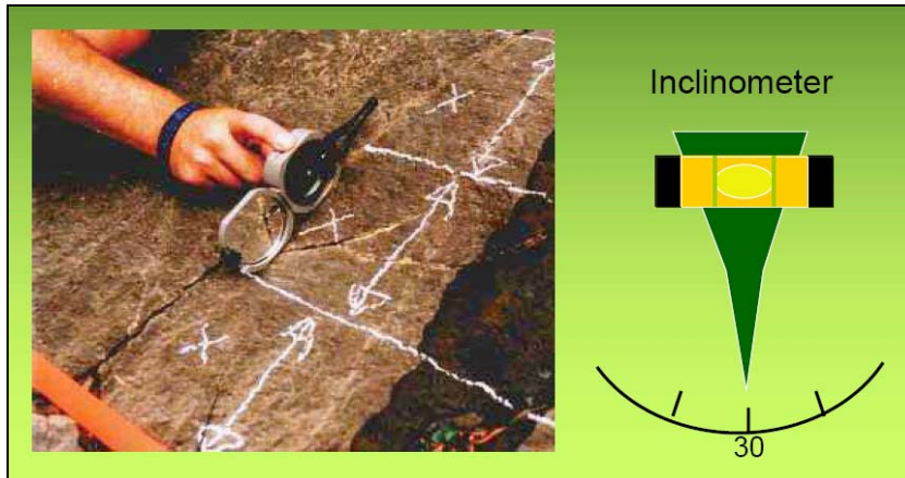
Figure 7.13. Dip angle measured by placing the long axis of the compass parallel with the dip direction. (Source: Boyce, 2006).
