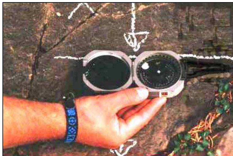
Figure 7.12. Strike is measured by placing the compass parallel with the outcrop face. (Source: Boyce, 2006).
