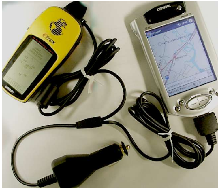
Figure 5.6. The system used to collect geological data in the field.
