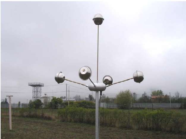
Fig. 2. Three axes antenna for electric field measurement in the frequency band [1Hz–100 kHz]. The instrumental sensitivity is equal to 1 \mu V / (m \sqrt{Hz}) .
