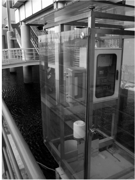
Fig. 3. The meteo-mareographic station (belonging to APAT RMN) in Genoa harbour.
