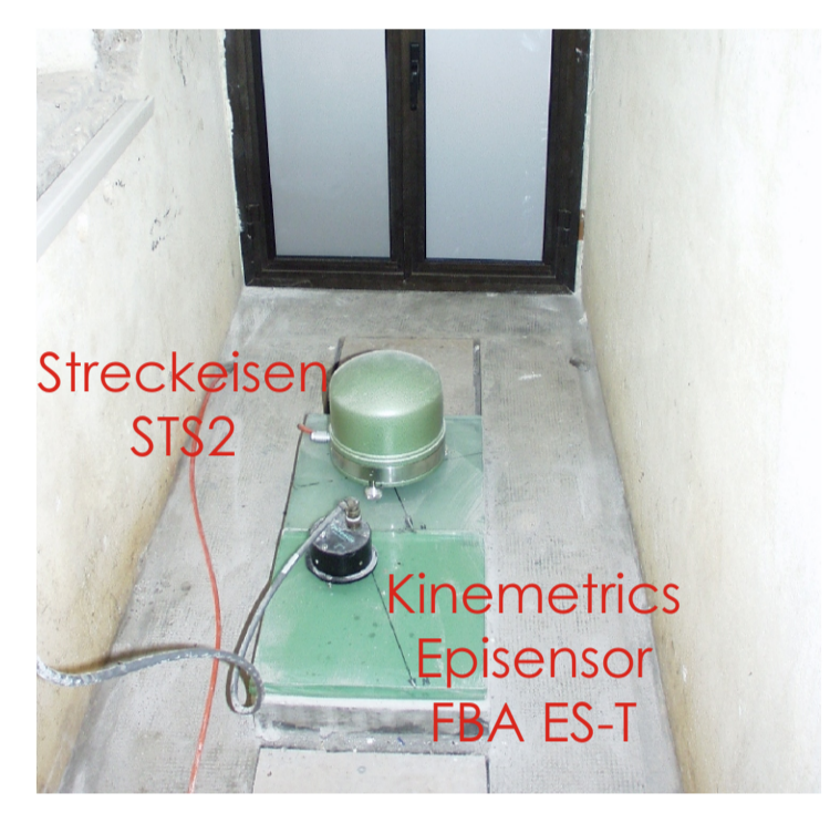
Fig. 2.3: Sensors at the broad-band station of Acomizza (ACOM).
