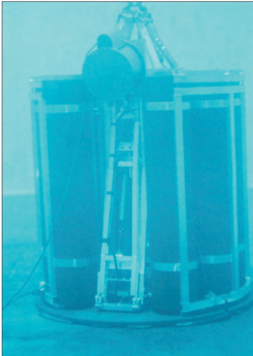
Fig. 1. The Pascal&Person three components ocean bottom seismometer. The syntactic foam provides buoyancy. A lever arm deploys the cylindrical seismometer array from the main structure.
