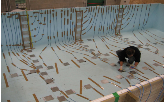
Fig. 1. Set up of one of the simulation tanks at L.A.R.A. laboratory. It is equipped with 160 electrodes.
