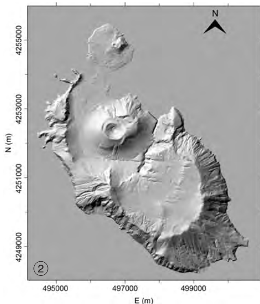
Fig. 2. Shaded relief image of the 10×10 m grid DTM of Vulcano Island.
