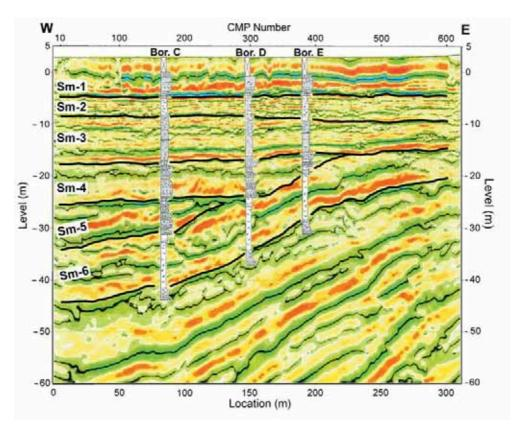
Fig. 12. Depth-converted S-wave seismic reflection profile across the Suminoe flexure combined with the boring survey result (vertical exaggeration  $\times$  4). See fig. 10 for the location of the survey line.
