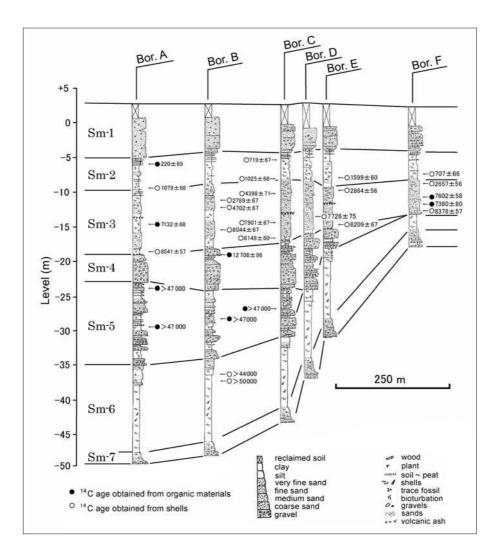
Fig. 11. Correlation of continuously cored boreholes across the Suminoe flexure in South Osaka. See fig. 10 for the location of each boring site. Modified from Nanayama *et al.* (2000a).
