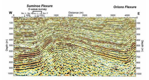
Fig. 10. Depth-converted *P*-wave seismic reflection profile across the Suminoe and Oriono flexures in south Osaka (vertical exaggeration  $\times$  2). See fig. 7 for the location of the survey line. Locations of *S*-wave reflection survey line and six boring sites are also shown on the profile.
