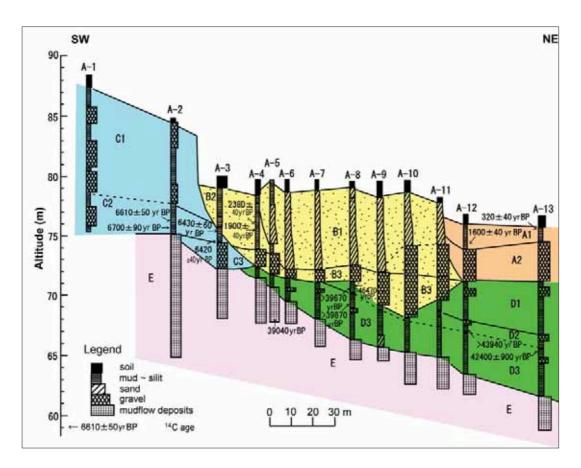
**Fig. 6.** Correlation of continuously cored boreholes within the flexure zone of the Fukaya Fault System in the Takasaki area. See fig. 4 for the projected location of the survey area. 5 stratigraphic units A-E are recognized, and each unit except for the unit E is divided into several subunits. After Mizuno *et al.* (2001).
