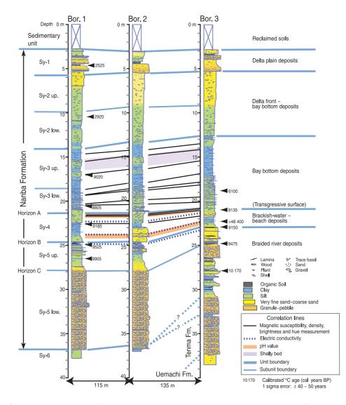
**Fig. 9.** Summarized stratigraphic correlation between boreholes 1, 2 and 3. The elevation of the three borehole sites is 2.5 m above the sea level. See fig. 8 for the location of each boring site. A clay bed intercalated at the depth of 33 m of borehole 3 is correlated to the Tenma Formation because it yields a pollen assemblage of the first half of the Last Glacial Stage. After Miura *et al.* (2002).
