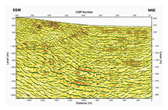
**Fig. 5.** Depth-converted seismic reflection profile for the Satomi line west of Takasaki (no vertical exaggeration). See fig. 2 for the location of the survey line.
