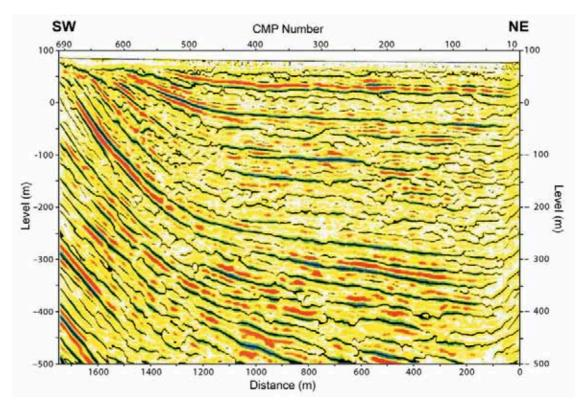
Fig. 3. Depth-converted seismic reflection profile for the Kaburagawa line to the south of Takasaki (vertical exaggeration  $\times$  2). See fig. 2 for the location of the survey line.
